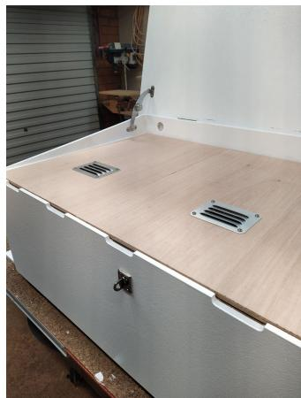
The tongue on the staple turns 90 degrees to lock the lid down and can be padlocked if thought to be necessary.
